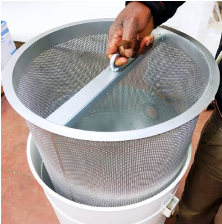
Liquids and solids separator
